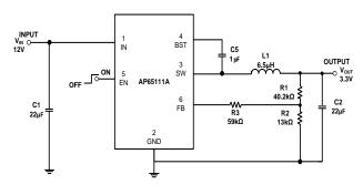
Figure 1. Typical Application Circuit
