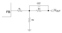
Figure 3. Feedback Divider Network
