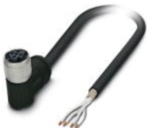
Sensor/Actuator cable, 4-position, PE-X halogen-free, black, shielded, free cable end, on Socket angled M12 SPEEDCON, A-coded, Cable length: 2 m, For railway applications
