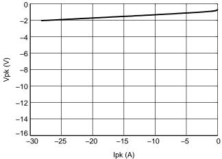
Figure 2. Negative TLP I-V Curve
