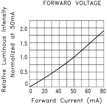
Fig.4 RELATIVE LUMINOUS INTENSITY VS. FORWARD CURRENT
