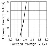
Fig.2 FORWARD CURRENT VS. FORWARD VOLTAGE
