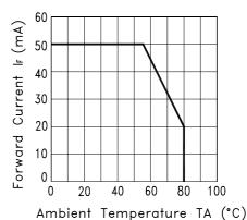
Fig.3 FORWARD CURRENT DERATING CURVE
