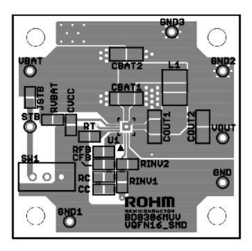
Figure 20. Assembly Layer
