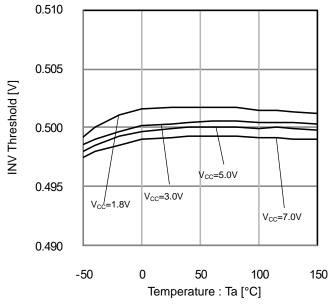
Figure 1. INV Threshold vs Temperature
