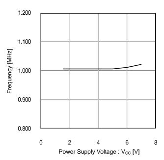
Figure 4. Oscillation Frequency vs Power Supply Voltage
