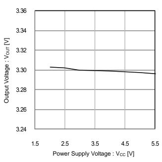
Figure 23. Output Voltage vs Power Supply Voltage (Output Current = 500mA)
