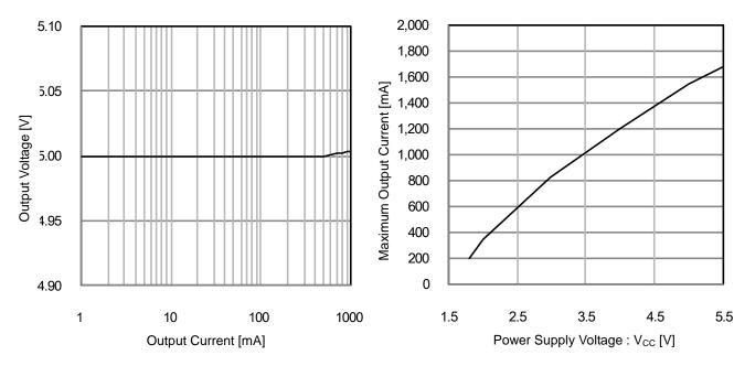
Figure 33. Output Voltage vs Output Current
