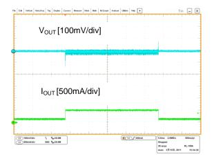
Figure 28. Output Current Response (Output Current = 100mA ⇔ 500mA 5msec/div)
