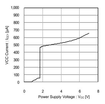
Figure 14. VCC Input Current vs Power Supply Voltage (V<sub>INV</sub>=0.8V, stop DC/DC)
