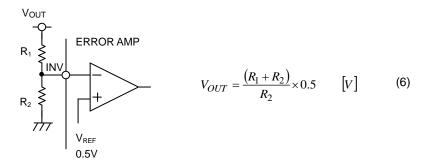
Figure 40. Setting of Feedback Resistance
