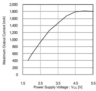
Figure 25. Maximum Output Current vs Power Supply Voltage
