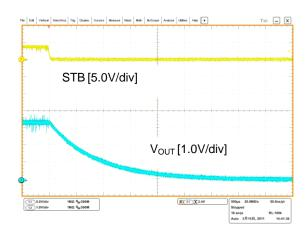
Figure 30. Discharge Waveform (STB: High to Low 500µsec/div)
