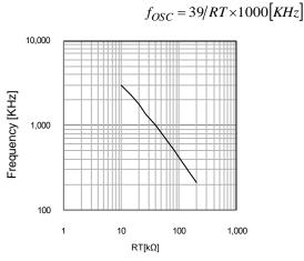
Figure 38. Oscillation Frequency vs RT Pin Resistance
