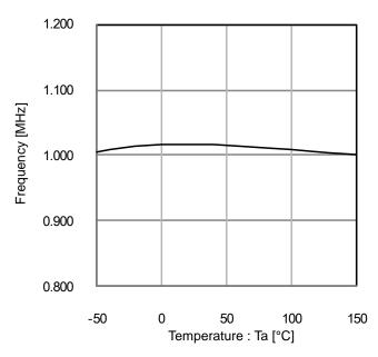
Figure 3. Oscillation Frequency vs Temperature
