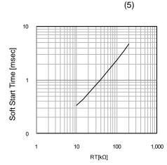
Figure 39. Soft-Start Time vs RT Pin Resistance
