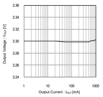
Figure 24. Output Voltage vs Output Current
