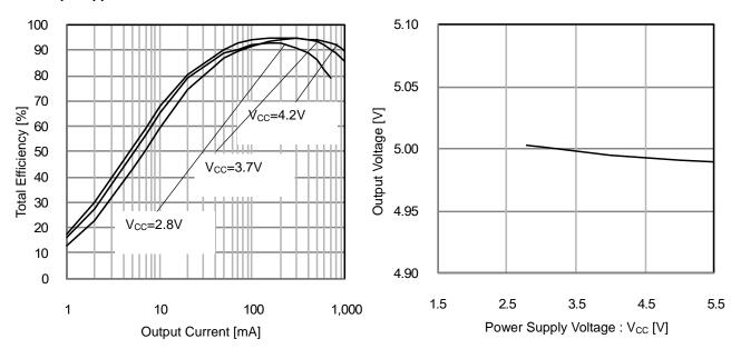
Figure 31. Total Efficiency vs Output Current (Power Conversion Efficiency)
