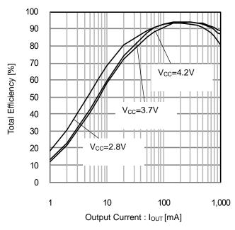
Figure 22. Total Efficiency vs Output Current (Power Conversion Efficiency)
