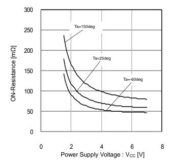
Figure 13. ON-Resistance vs Power Supply Voltage (LX2 Nch FET)
