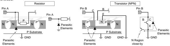
Figure 44. Example of monolithic IC structure
