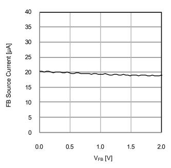
Figure 8. FB Source Current vs  $V_{FB}$  ( $V_{INV}$ =0.2V)
