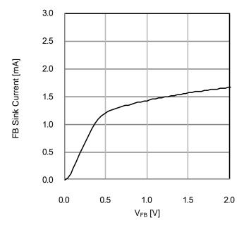
Figure 7. FB Sink Current vs  $V_{FB}$  ( $V_{INV}$ =0.8V)
